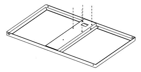
STEP 2: Place up to six (6) concrete blocks as shown below (mount not shown for clarity).
